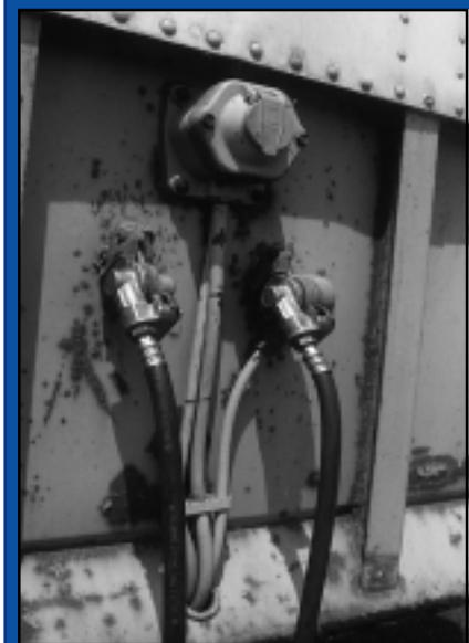
***Designers reduced corrosion by eliminating entrapment areas where moisture and poultrice can be trapped or retained; they reduced the number of sharply angled meeting surfaces, “dead ends” and narrow openings; and they closed unneeded holes in body panels and provided better drainage.***
