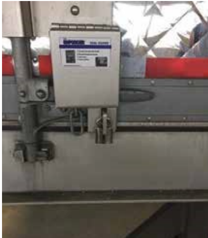
Transport Security's Enforcer Seal Guard Lock is a hasp and trailer seal protector designed to prevent unauthorized seal removal and tampering while in transit. The self-contained lock is made from hardened steel and has a corrosion-resistant stainless-steel surface. It is engineered to be mounted onto existing trailer latches.
