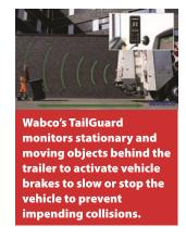
TailGuard monitors stationary and moving objects behind the trailer – such as pedestrians, vehicles, cargo and infrastructure - to activate vehicle brakes to slow or stop the vehicle to prevent impending collisions. Sensors mounted to the trailer monitor an approximately 6-foot radius and activate if the brakes are not applied within two or more feet of the object.
