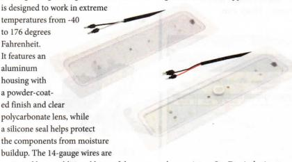
protected by an additional layer of the company's proprietary Sta-Dry jacketing to guard against corrosion, and male 0.180-bullet connectors on the wires help simplify installation. A passive infrared motion sensor turns on the dome lamp when activity is detected, and the lamp will shut off automatically after five minutes of inactivity.
