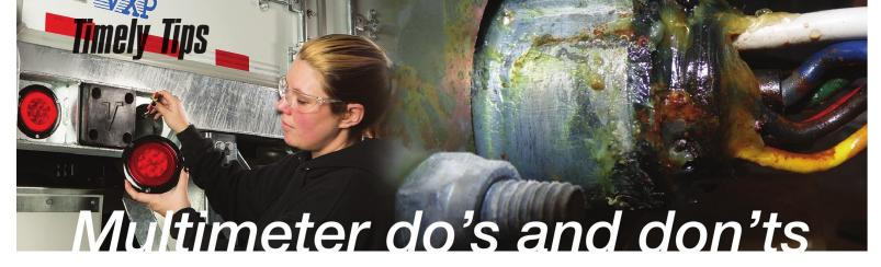
As the spring season starts to thaw winter's freeze, it's a good time to give your trucks and trailers a good once-over to ensure that all components are operating properly. The lighting system is a good place to start. Check for any loose connections, broken wires or excessive corrosion at the connections, since, of course, any electrical device needs power to work. A multimeter is your go-to tool for troubleshooting a circuit or electrical device.
