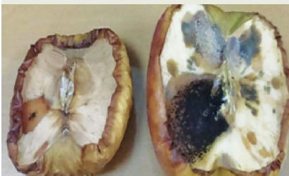
The apple sample on the left was stored in a refrigerator and exposed to the Light-Shield LED, while the sample on the right was exposed only to standard LED lighting.
