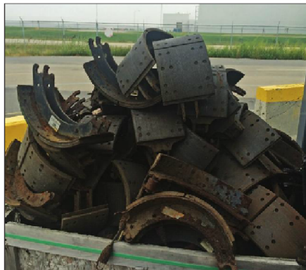
When left unchecked, corrosion can wreak havoc throughout a tractor and trailer, specifically electrical and braking systems as shown above.
