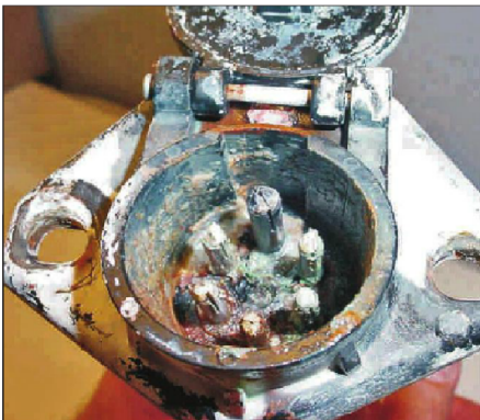
When left unchecked, corrosion can wreak havoc throughout a tractor and trailer, specifically electrical and braking systems as shown above.
