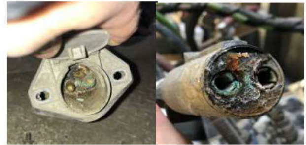
Dual Pole Socket Corrosion
