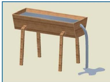
Now imagine the hole is 12" from the top of the trough with a potential energy of 12V. The deeper the hole, the more pressure is exerted from the great amount of water.
