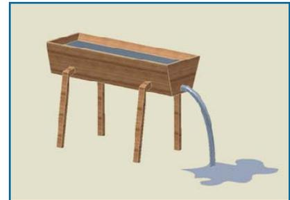
The difference in height, causes a difference in the amount of water pressure escaping the hole, this pressure represents VOLTAGE. So, the higher the potential water pressure, the more force the water is able to exert and the more likely it is to flow through the hole to the ground.
